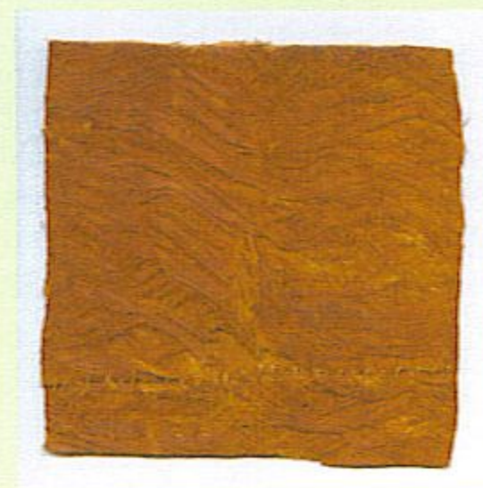
Fig. 1: Plastic-reinforced fibre from the renewable sub-bark of Ficus natalensis
