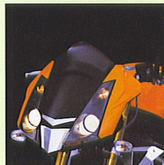
Fig. 2: Motor cycle front fairing made from polyurethane
