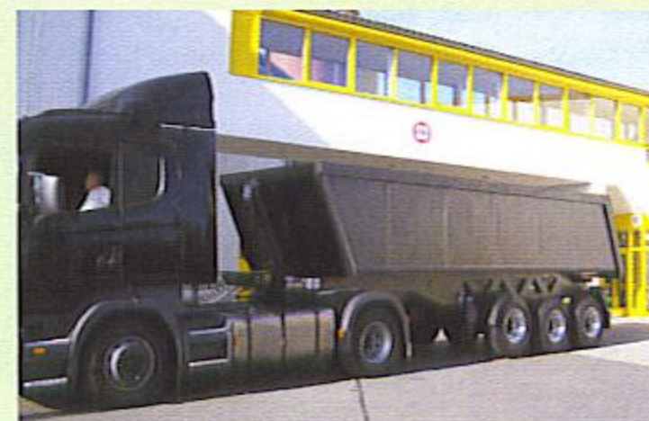
Fig. 3: Saddle cover made from wool hair reinforced epoxy resin
