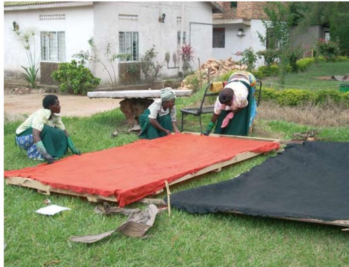
9. The finished cloth is stretched out on a frame. It is then laminated on a non-woven backing in order to create a high-quality wallcovering.
